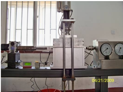
图 2 大型剪拔仪 Fig.2 Large scale direct shear- pullout apparatus
